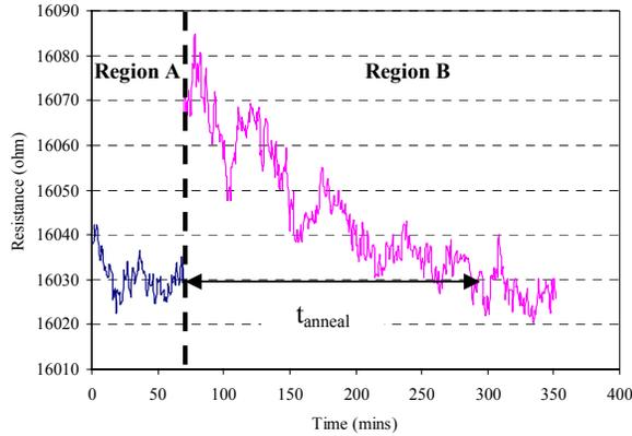
Figure 8. One example of the annealing process. It shows the observed response of the sensor when we burn the sensor with 100 $\mu\text{A}$  after the introduction of 10-sec dose of 50ppth alcohol vapor. We recorded the annealing time ( $t_{\text{anneal}}$ ) from this graph.
