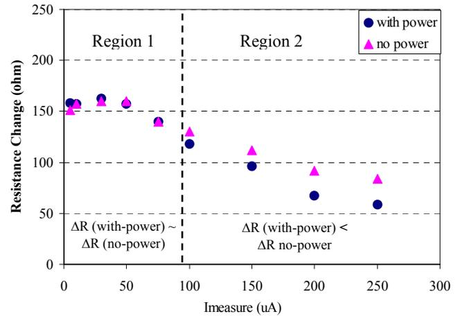
Figure 10. Response of the sensor with different  $I_{\text{measure}}$ . We have also compared its behavior on cases of “with power” and “no power”. Overheat effect of the MWCNTs definitely has influence on the sensors’ response towards the alcohol vapor.
