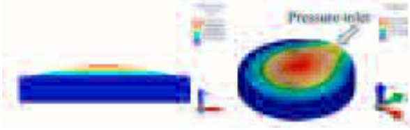
Figure 5: FEM [side and 3D view] using Algor to simulate the deflection of the whole diaphragm. The scale of the deformed shape is 5 percent of the model size. The maximum deflection under varying pressure is plotted in Figure 6.
