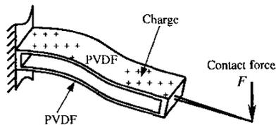
Fig. 3. Illustration of the parallel beam structure.
