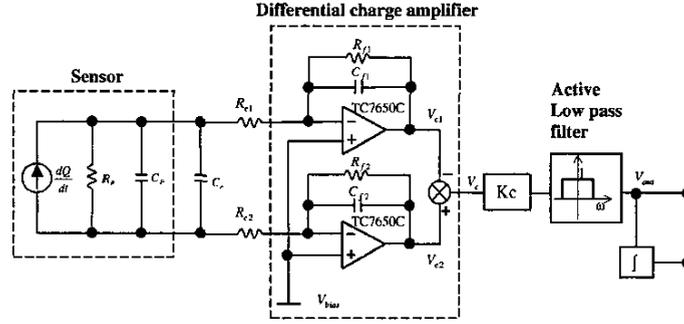
Fig. 4. Schematics of the electronic circuit.
