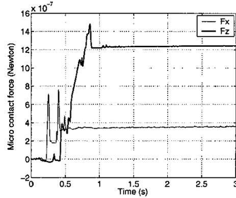
Fig. 7. 2-D sensor responses when force exerting along  $75^\circ$  with respect to the ZY plane.
