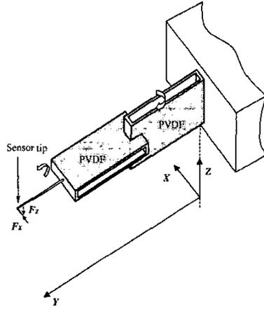
Fig. 2. Illustration of the 2-D force sensor.
