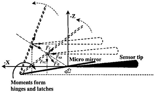
Fig. 9. Illustration forces acting on a micro mirror during lift-up process.
