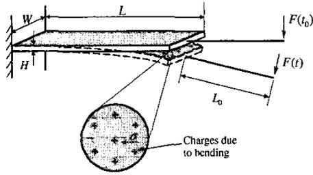
Fig. 1. Illustration of the force sensor using 1-piece PVDF film.
