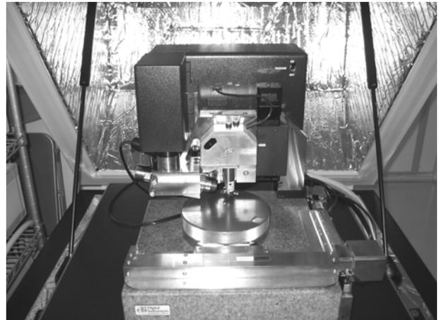
Fig. 5. Atomic Force Microscope employed for experiment
