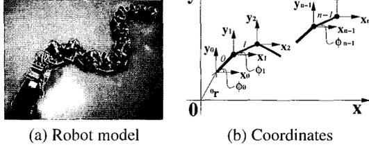
Fig. 1: Model of the snake-like robot and coordinates located on the robot
