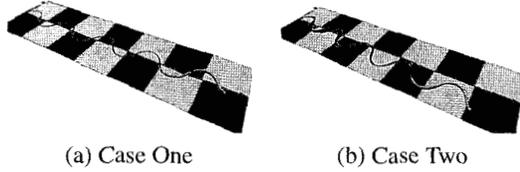
Fig. 4: Creeping locomotion of the snake-like robot on two different environments
