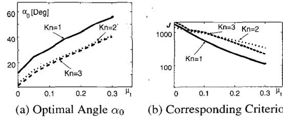
**Fig. 9: Optimal winding angle  $\alpha_0$  and corresponding performance criterion, while  $K_n = 1$ ,  $K_n = 2$ , and  $K_n = 3$**
