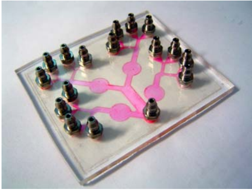
Figure 9. Photograph of the SU-8 channels on the PMMA substrate of the microfluidic system with parallel sample preparation capability.
