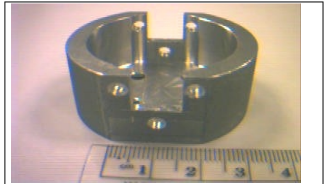
Figure 5. A 2cm center-to-sensor disk.
